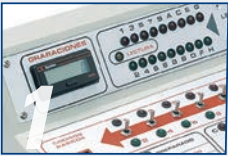
READING INDICATOR AND KEY CODE VISUALISER
