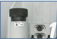
COPYING INDEX WITH MICROMETRIC ADJUSTMENT
