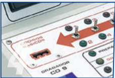
SWITCHES FOR SELECTION OF BASIC CODES
